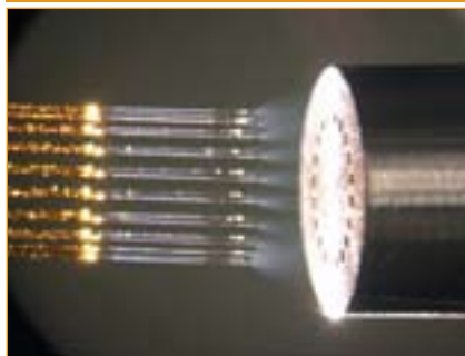
FIGURE 10. Multi emitter ESI source provides 10-fold increase in ion production
